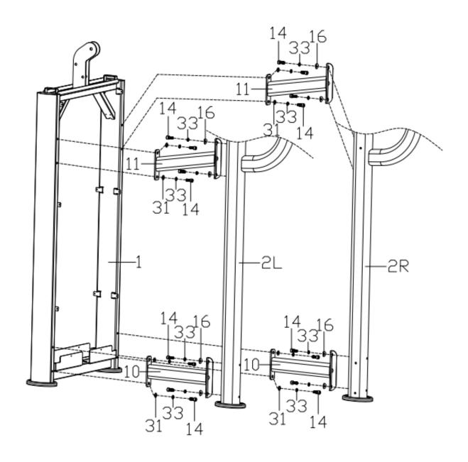
Use hexagon cylindrical head bolts (14), spring washers (33), and flat washers (31) to pre-lockthe side of below transverse tube frame (10) and side of upper transverse tube frame (11) to the counterweight frame (1), note that the hexagonal cylindrical head bolt (14) is not locked first;
