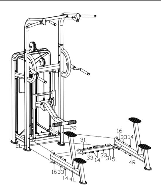
Use hexagon cylindrical head bolts (14), spring washers (33) and curved washers (16) to pre-lock the front support frame (4L/R) on the below upright tube frame (2L/R) respectively;
