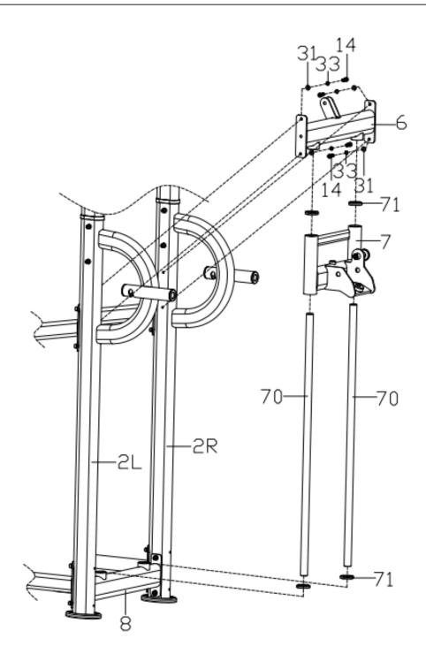
Insert the bottom two buffer pad (71) into each of the two slide rods (70), then insert the two slide rods (70) into the hole of the below transverse tube frame(8), and insert adjustable frame (7), buffer pad (71), middle transverse tube frame (6)in sequence;
