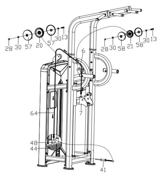
First move the adjustable frame(7) to the highest point and fix it, then lock the bolt at either end of the wire rope (64) to the adjustable frame (7), and the other end of wire rope(64) is installed by winding the rope in the direction of the arrow;
