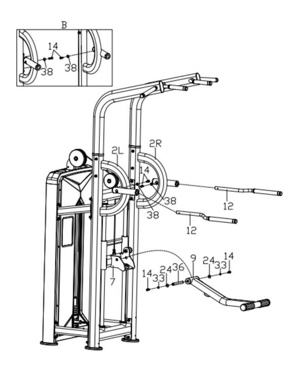
Use the hex cylindrical head bolt (14) and stainless steel sleeve (38) to lock the press handle (12) to the below upright tube frame(2L/R), note that the direction of hex cylindrical head bolt (14)(as shown in Figure B below), if it is reversed, the press handle(12) is unavailable;
