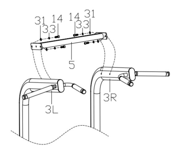
Use hexagon cylindrical head bolts (14), spring washers (33), and flat washers (31) to lock the upper transverse tube frame (5) on the upper upright tube frame (3L/R);
