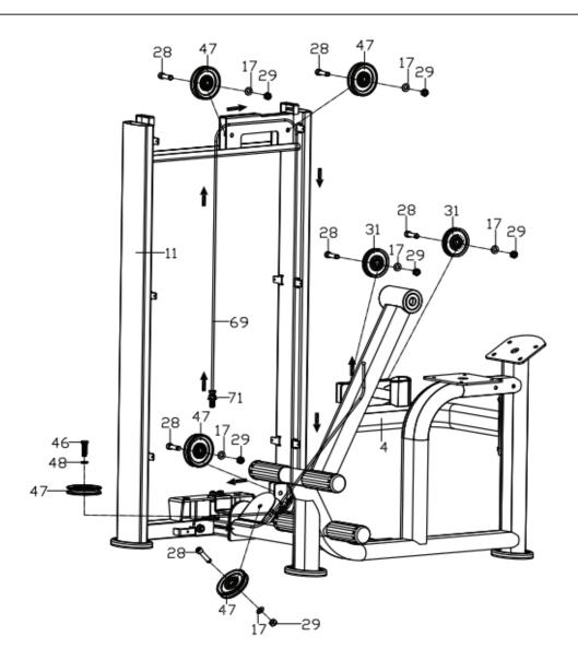
Wrap one end of the wire rope (69) in the direction of the arrow;
