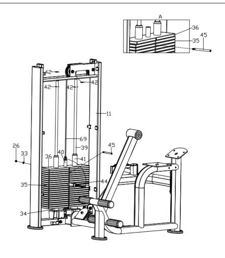
First, the buffer pad (34), slide rod (39), weight block (35), guide block (36) are loaded into the weight frame (11) in order;
