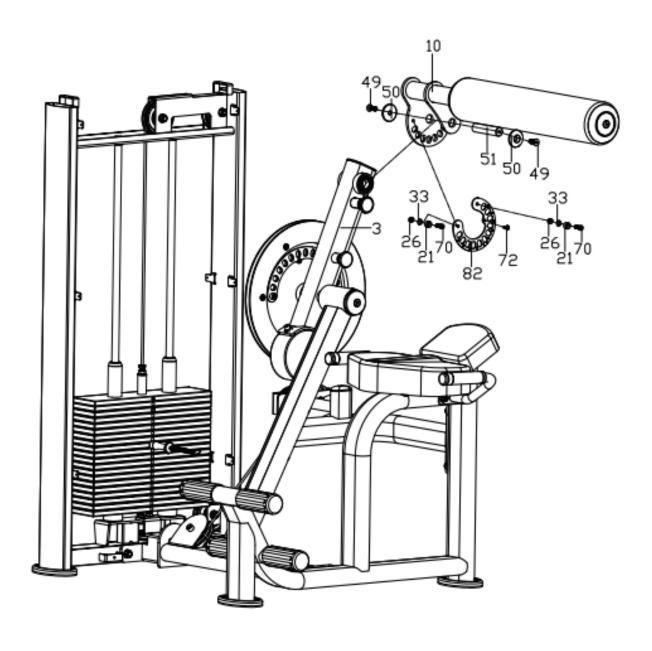
First, insert the foam frame(10) into the swing frame (3), and use the hex countersunk head screw (49), the end cap(50), connecting shaft (51) to lock tightly;
