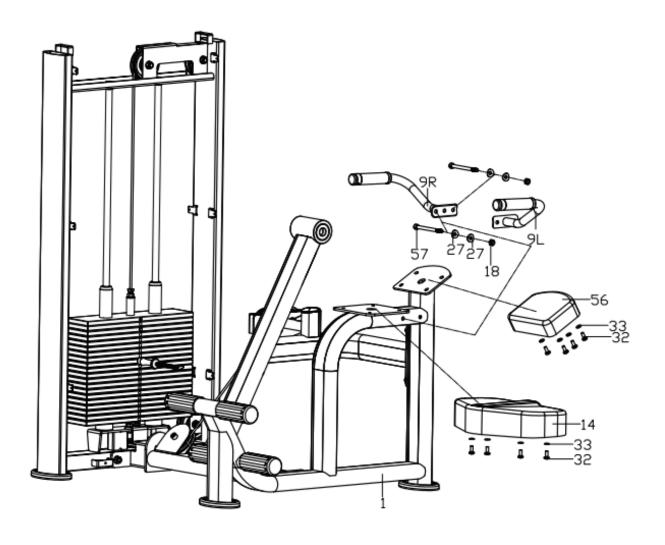
First,lock to the left and right fixed handles (9L/R) to the rear support frame(4) with hexagon cylindrical head bolt (57), arc washer (27), nylon nut (18) tightly;
