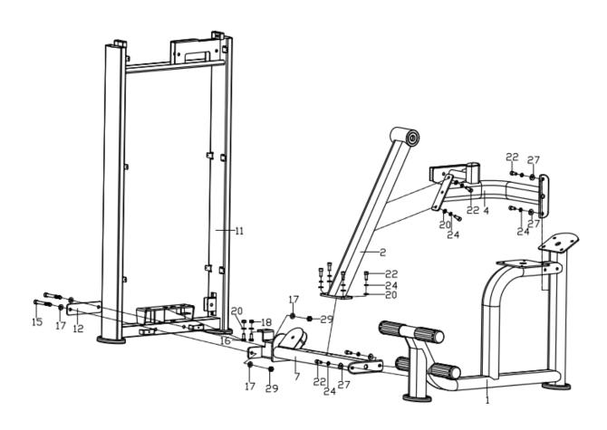
Prelock the connect frame (7) to the main base frame (1) with the hex cylindrical head bolt (22), spring washer (24) and arc washer (27);
